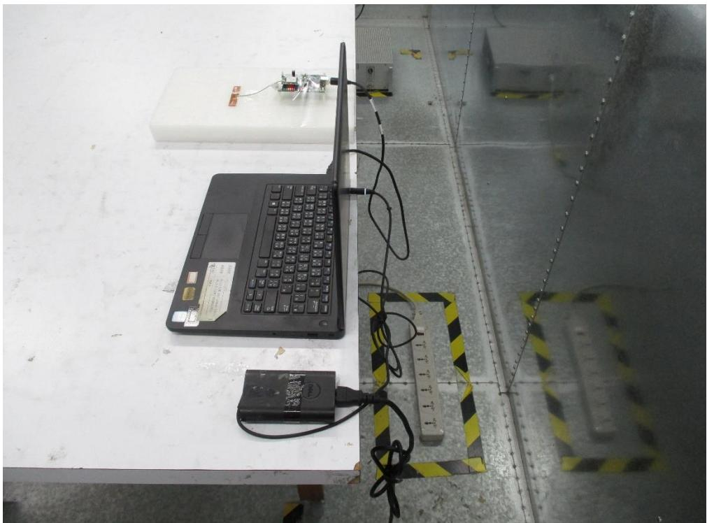
**Radiated Emission Below 1GHz Test**
