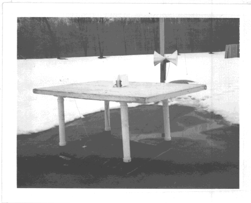
Figure 5.4. DUT on the open-site test table.
