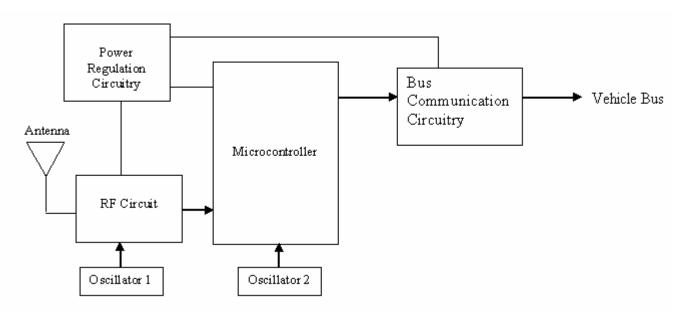
oscillator circuit 1 is at 9.5094 MHz and oscillator circuit 2 is at 8.00 MHz.
