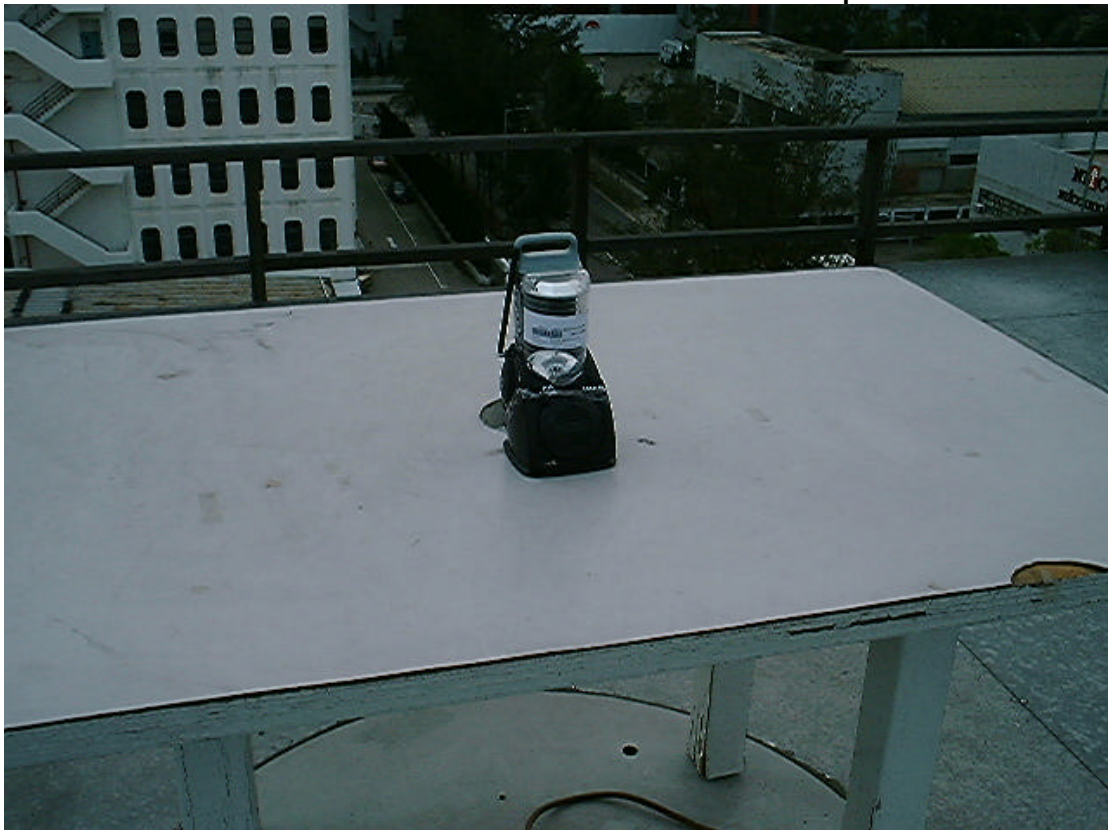
Measurement of Radiated Emission Test Set Up
