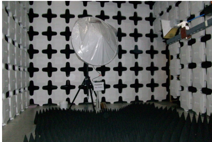
Ridge-Guide Horn Antenna (1GHz to 18GHz)
