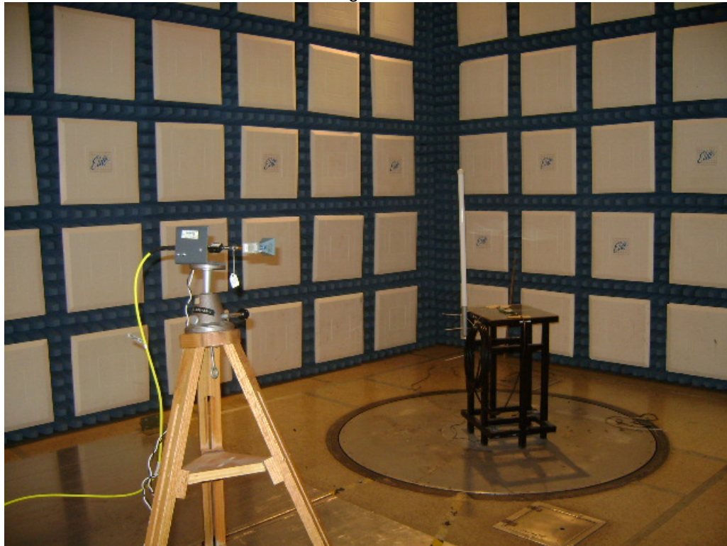
Test Setup for Radiated Emissions, 12dBi gain antenna – 18GHz to 25GHz, Horizontal Polarization
