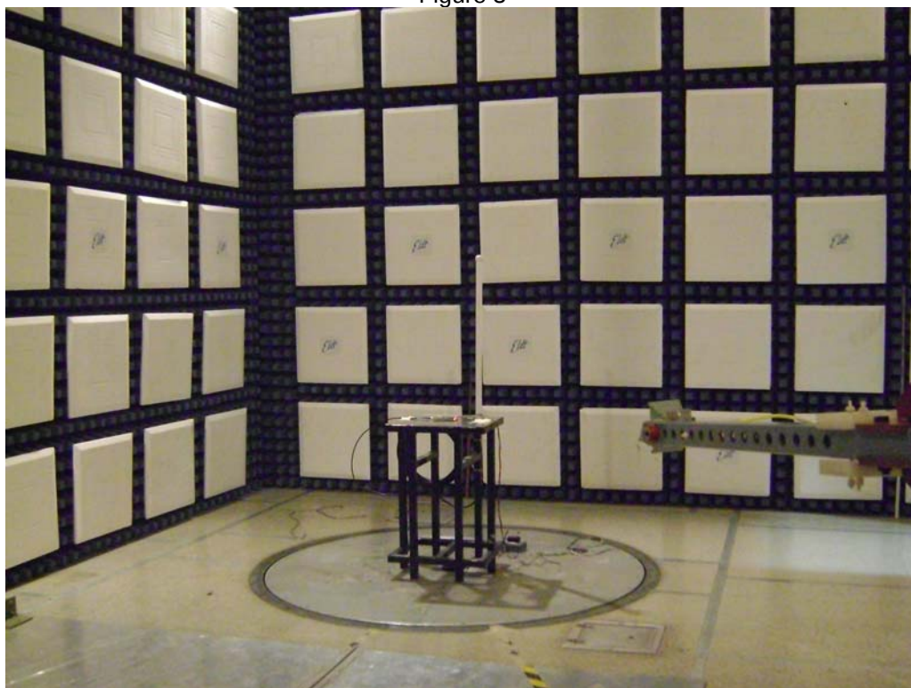
Test Setup for Radiated Emissions, 12dBi gain antenna – 2GHz to 18GHz, Horizontal Polarization
