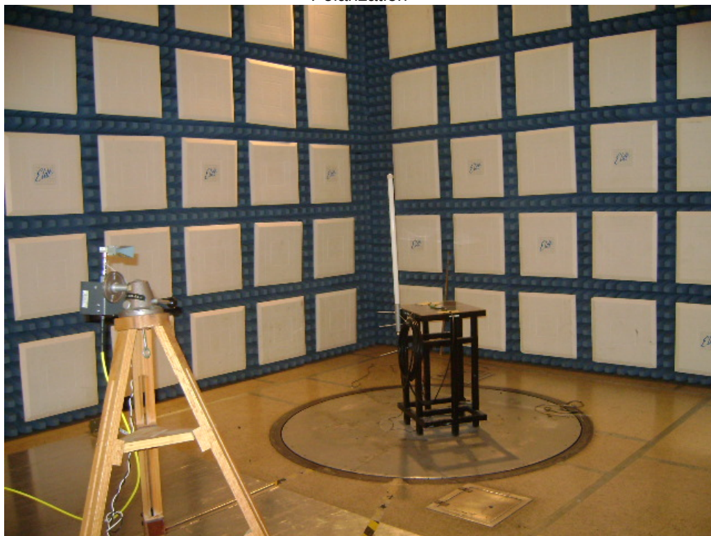
Test Setup for Radiated Emissions 12Bi gain antenna – 18GHz to 25GHz, Vertical Polarization
