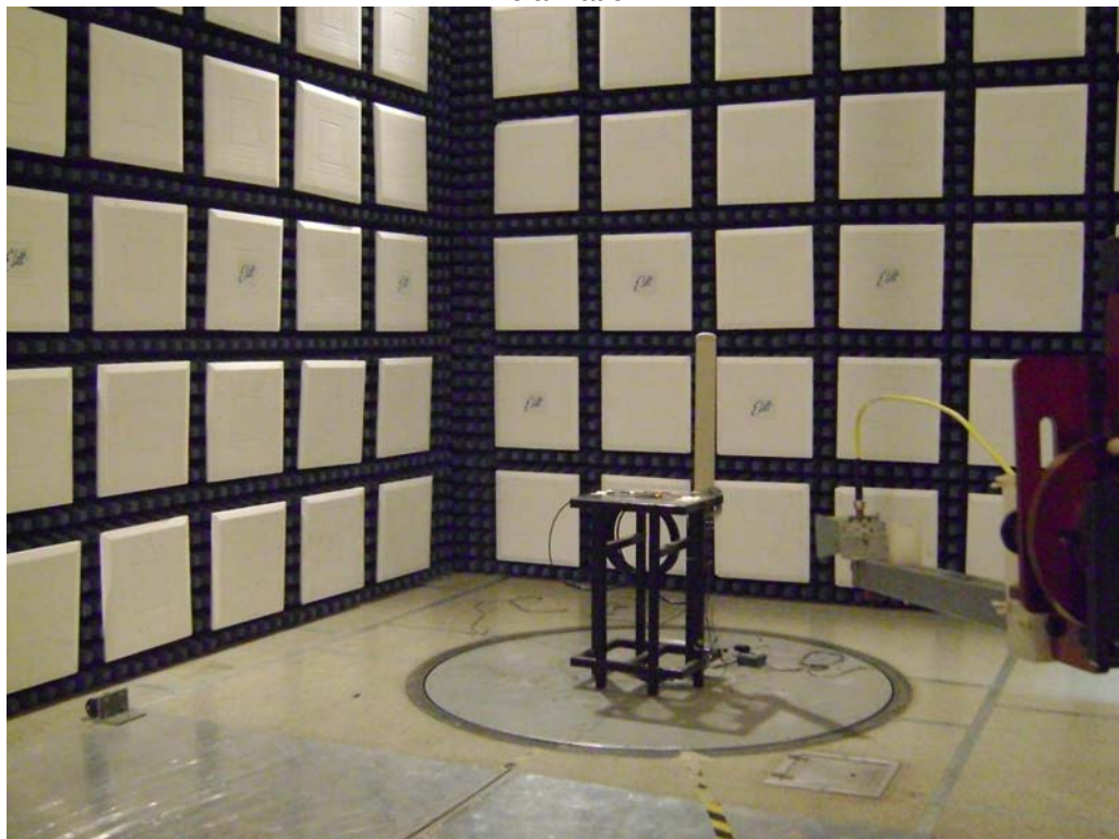
Test Setup for Radiated Emissions 15dBi gain antenna – 2GHz to 18GHz, Vertical
