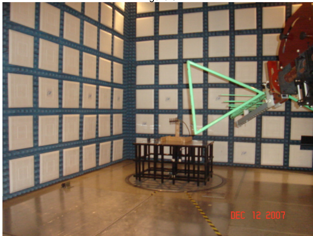
Test Setup for Radiated Emissions Yagi Antenna – Horizontal Polarization
