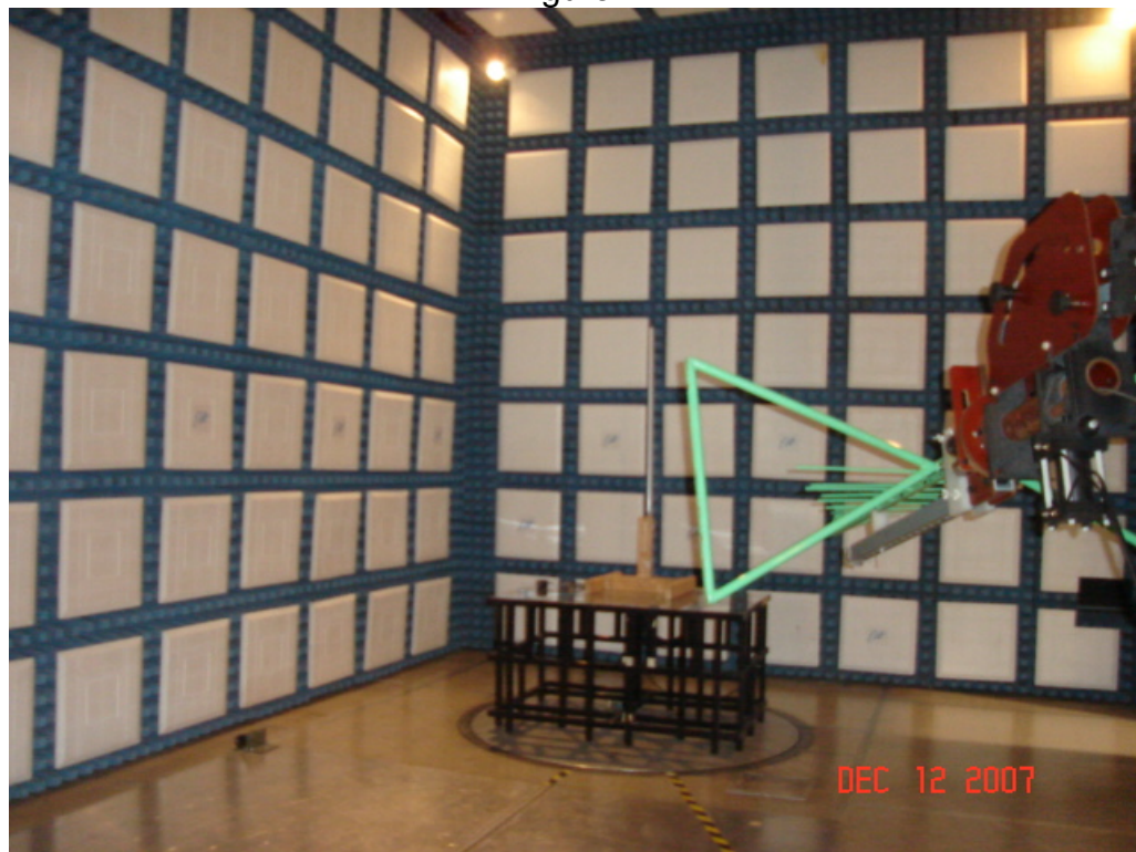
Test Setup for Radiated Emissions Omni Antenna – Horizontal Polarity
