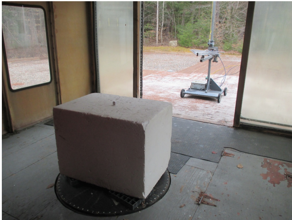
Test Setup, 200 MHz to 1 GHz, Horizontal Antenna Polarization
