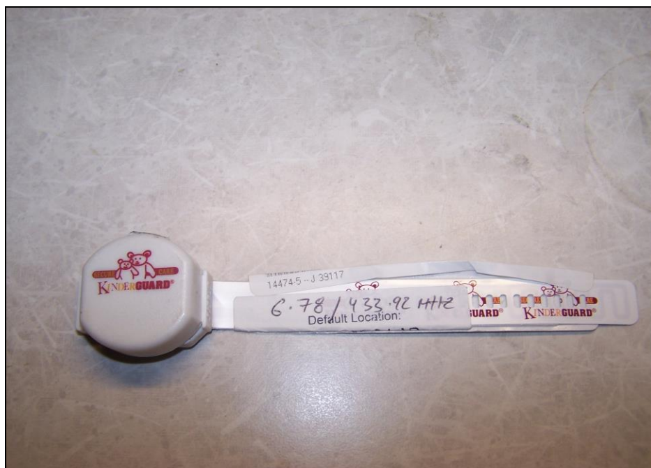
Photograph 1. Secure Care Products, 6.78 MHz Tag
