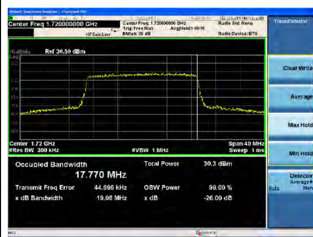
LTE Band 66, 16QAM, 20MHz-Low CH
