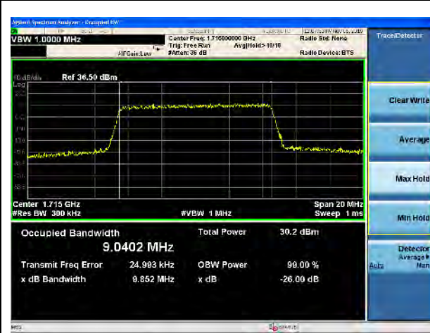
LTE Band 66, 16QAM, 10MHz-Low CH
