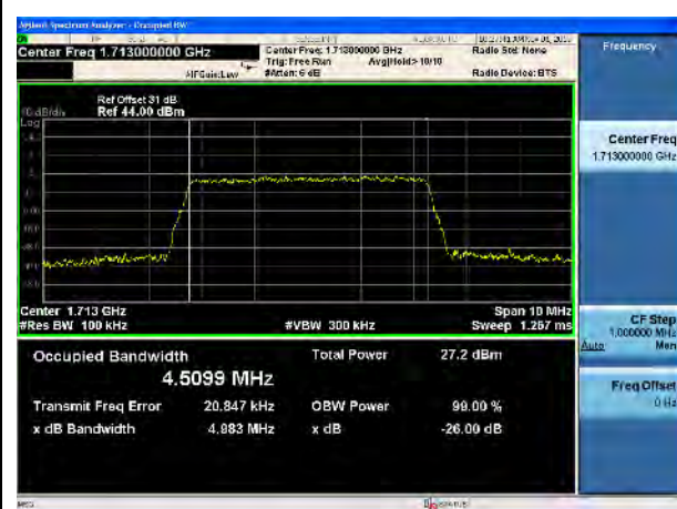
LTE Band 4, 16QAM, 5MHz-Low CH
