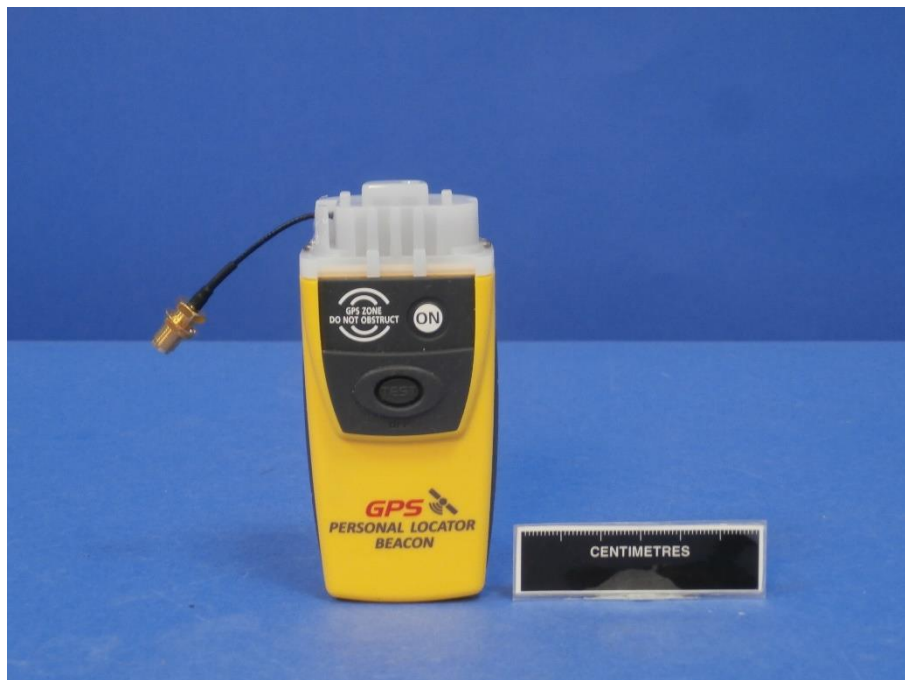
Modified Test Sample - 50Ohm conducted output
