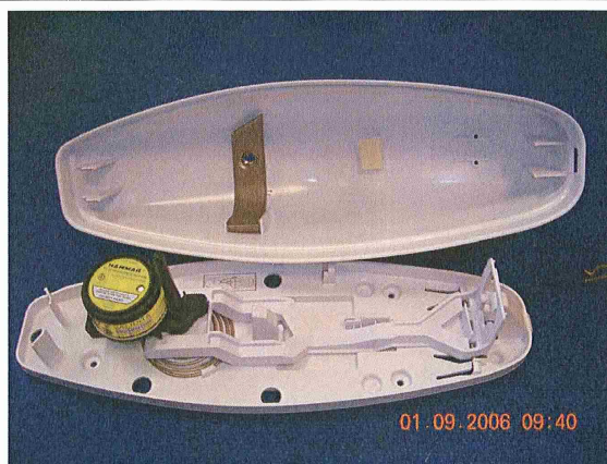
The G5 Float-Free housing, opened to show mechanism.
