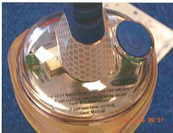
The G5 EPIRB beacon, Top view showing retroreflective material and self-test button.
