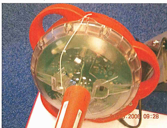
Top view of the C1 EPIRB/S-VDR capsule.
