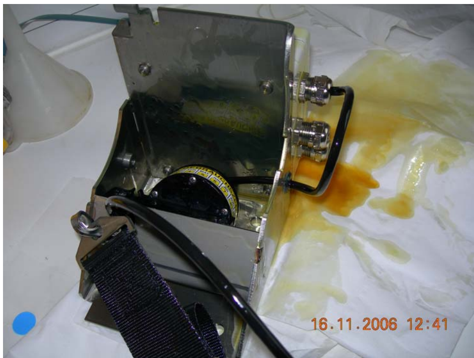
The C1 Float-Free bracket (cover removed), no degradation was noted on any components.
