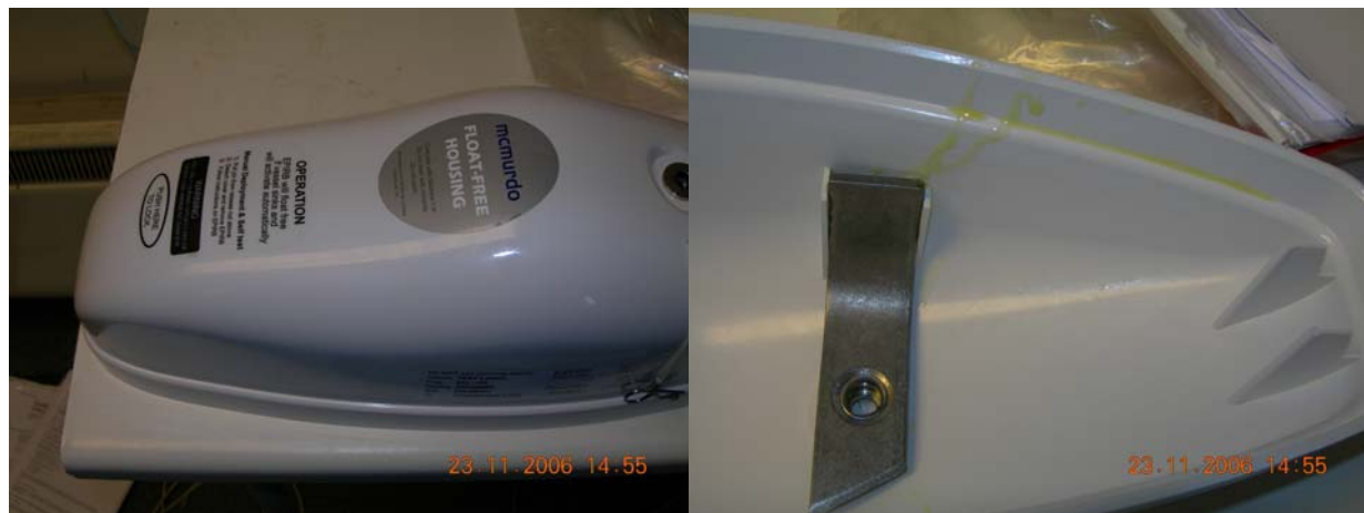
Inside and outside views of Float-Free housing cover (cleaned). No degradation was noted on any part.
