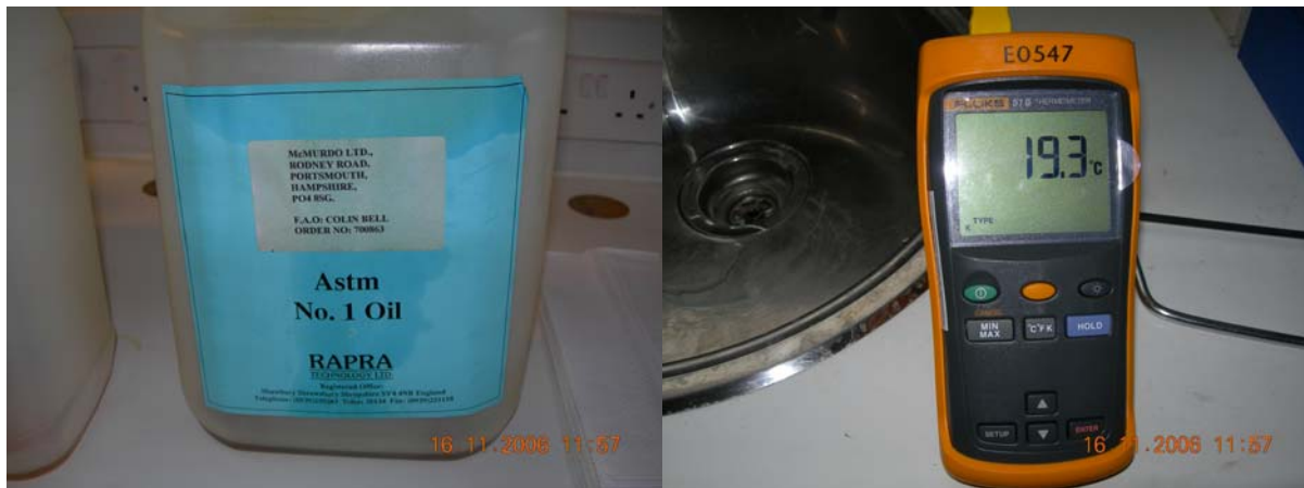
The Oil grade and supplier and the temperature of the oil at the end of 3 hour test.
