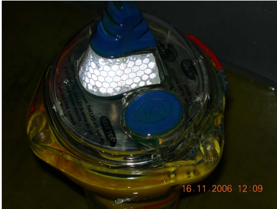
Close-up of the G5 EPIRB beacon, before washing – no degradation was seen except slightly in the Retroreflective tape which is a pre-approved component and bears its own wheelmark.
