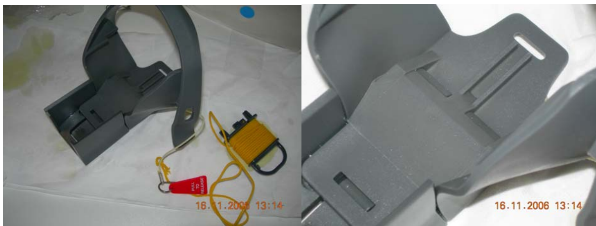
The G5/E5 manual Bracket assembly and Lanyard (cleaned) – No degradation was noted
