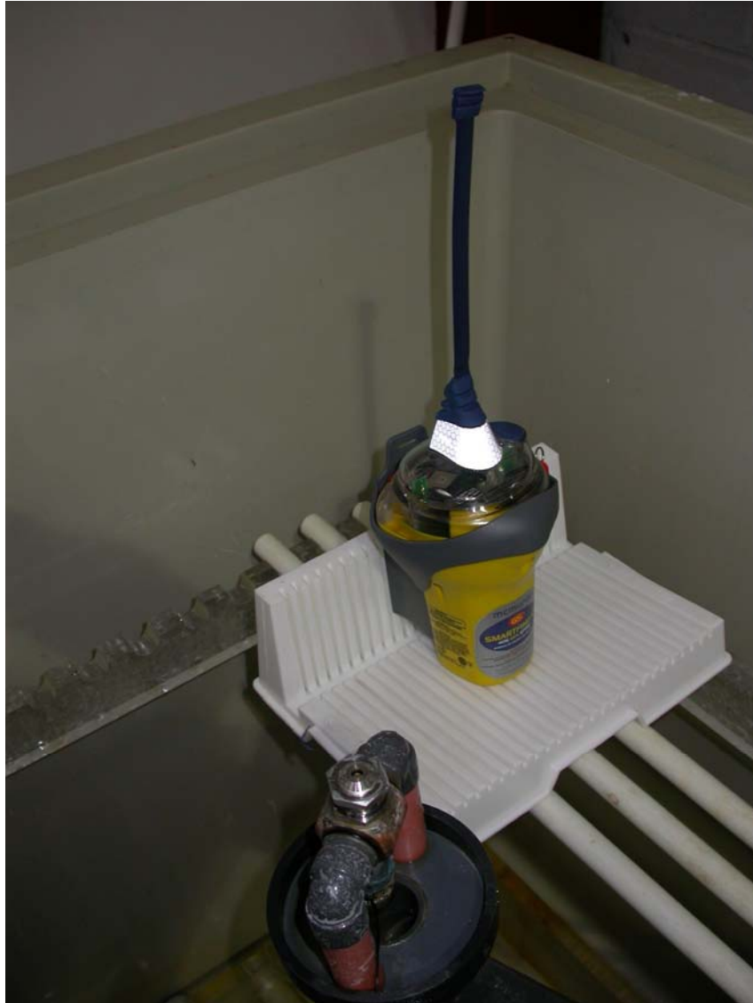
Photograph showing EUT in Manual Mounting in Salt Fog Chamber
