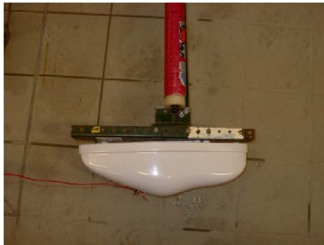
EPIRB mounted on the plunge pole ready test, Horizontal. - Pitching Cover down.
