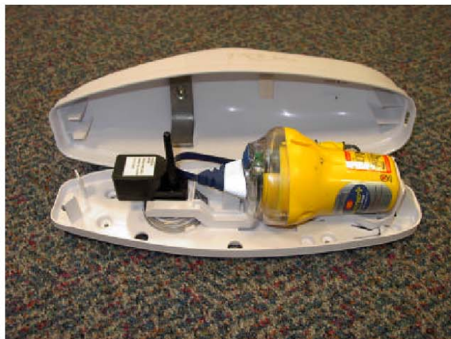
EPIRB mounted on the plunge pole ready test, Horizontal. - Pitching Cover down.
