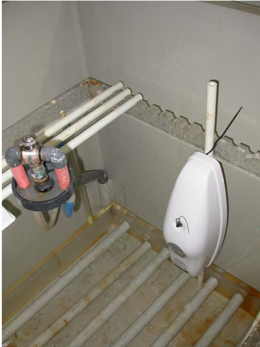
Photograph showing EUT in Float Free Mounting in Salt Fog Chamber
