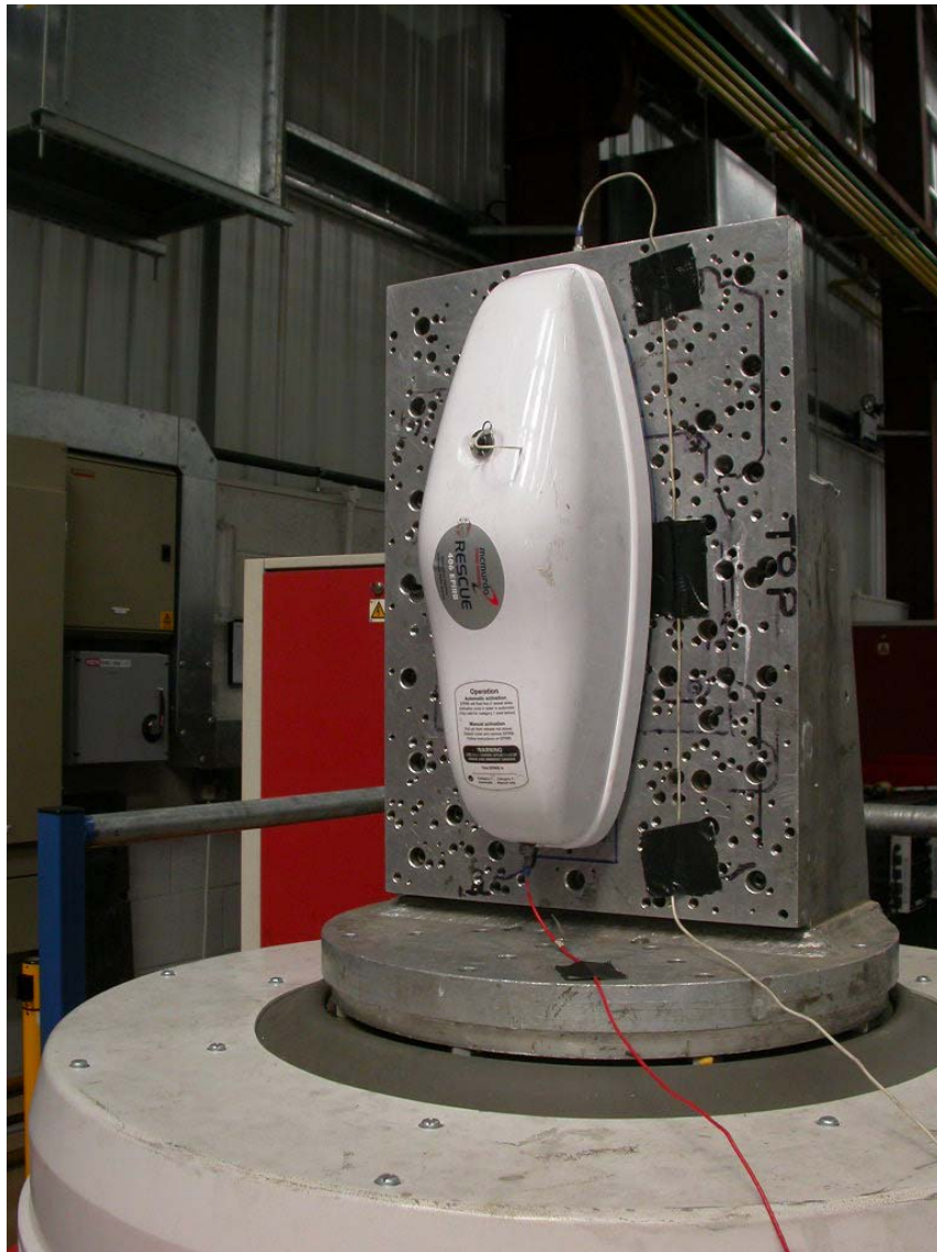
Photograph showing Ruggedness Test Set-up in Float Free Enclosure
