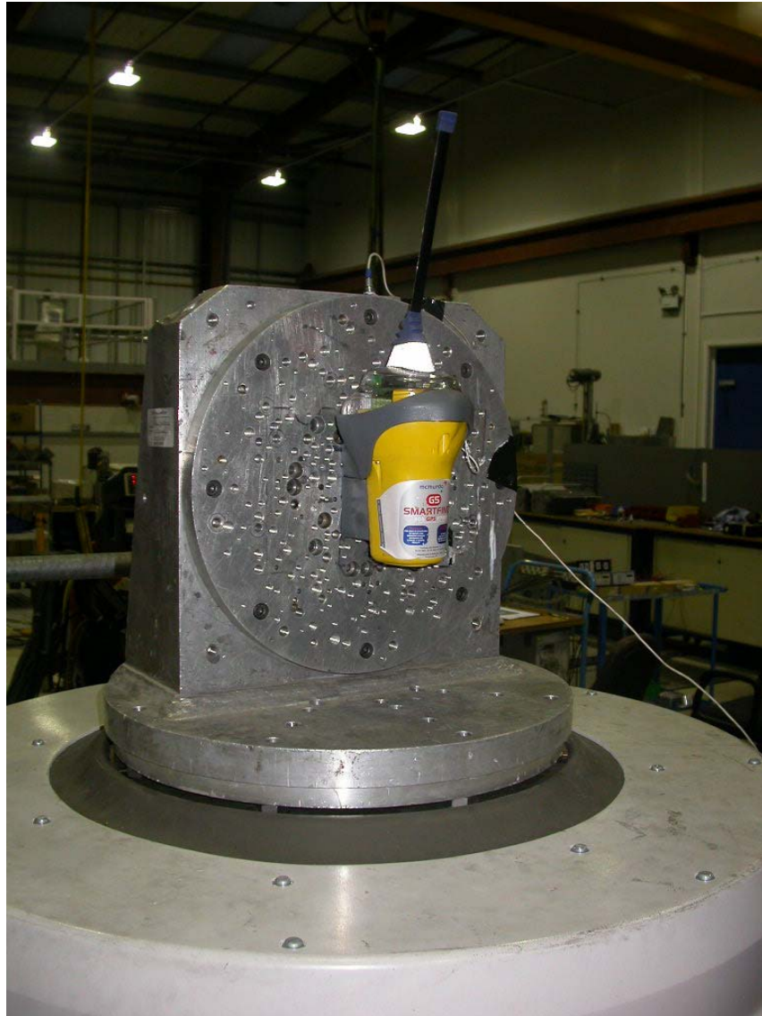
Photograph showing Ruggedness Test Set-up in Manual Release Bracket
