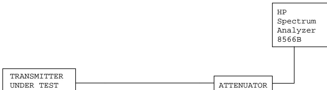
METHOD OF MEASUREMENT: The procedure used was TIA/EIA-603 STANDARD without any exceptions. The measurements were made using the shielded room located at TIMCO ENGINEERING INC. 849 STATE ROAD 45, NEWBERRY FLORIDA 32669.
