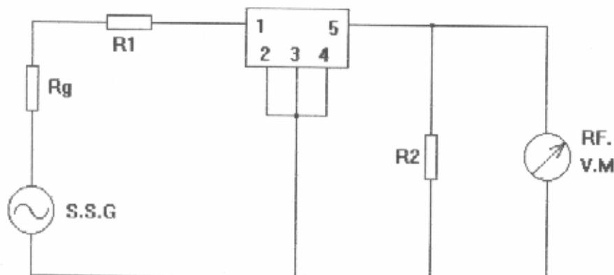
$R_g + R_1 = R_2 = \text{Input/Output Impedance}$
