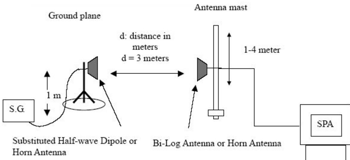
**Test procedure below 30 MHz**
