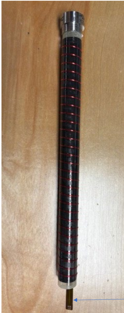
Silicon Steel Core Tube Wound with Magnet Copper Wire ('Antenna')
