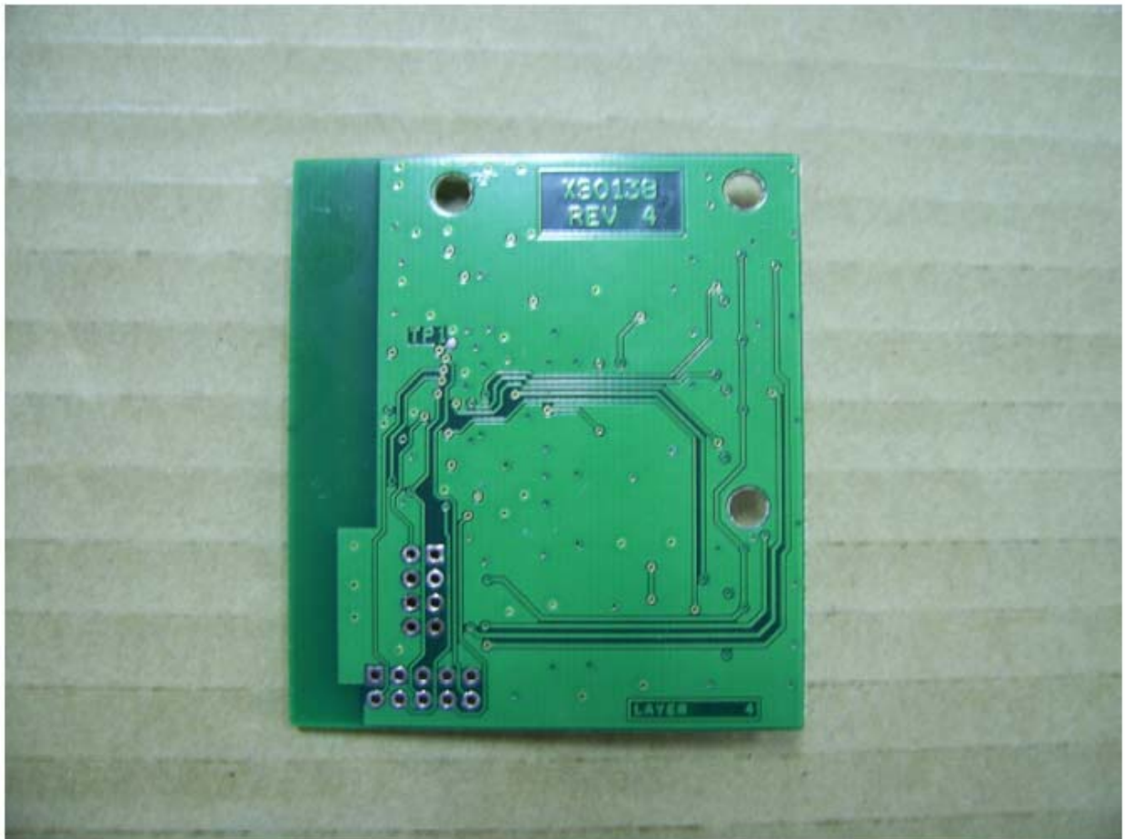
Figure 2: Internal – Back View – Z-Wave Board
