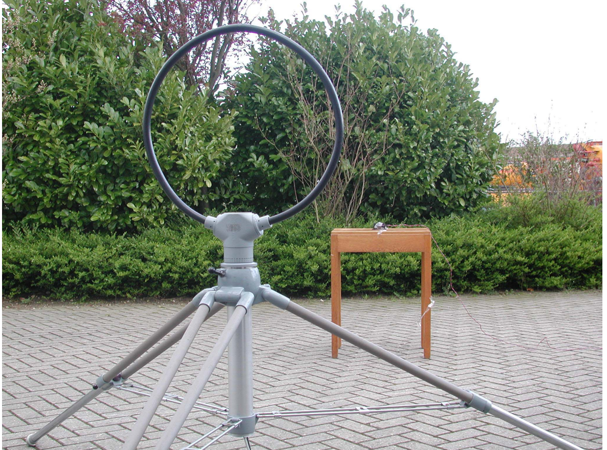
Photograph 5: 3 m test set up, ( < 30 MHz)
