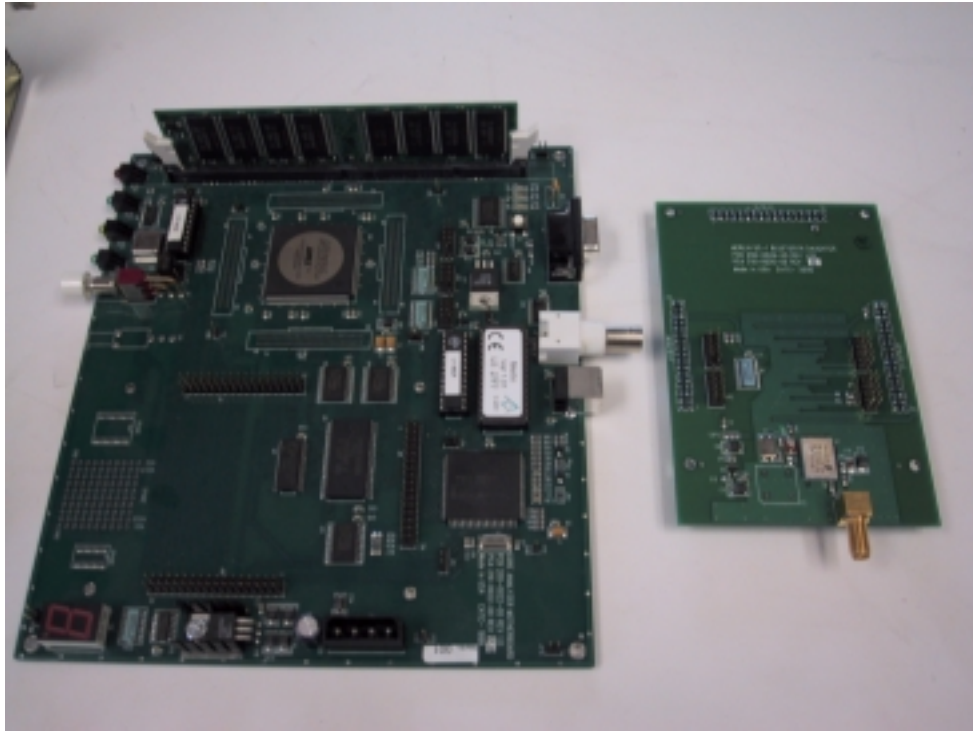
Main PCB / Radio PCB – Top View
