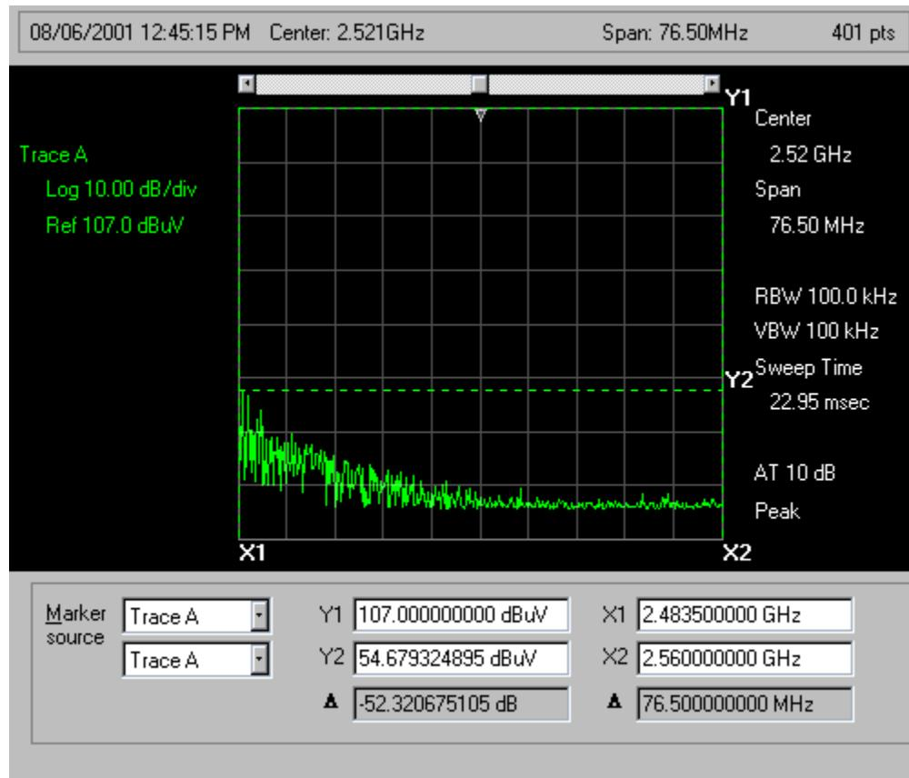
Note: No significant emissions were detected in any other Restricted Bands up to 24 GHz.
