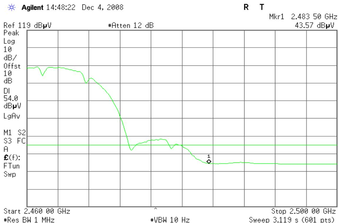
**Band Edges (IEEE 802.11g / CH Low)****Detector mode: Peak****Polarity: Vertical**
