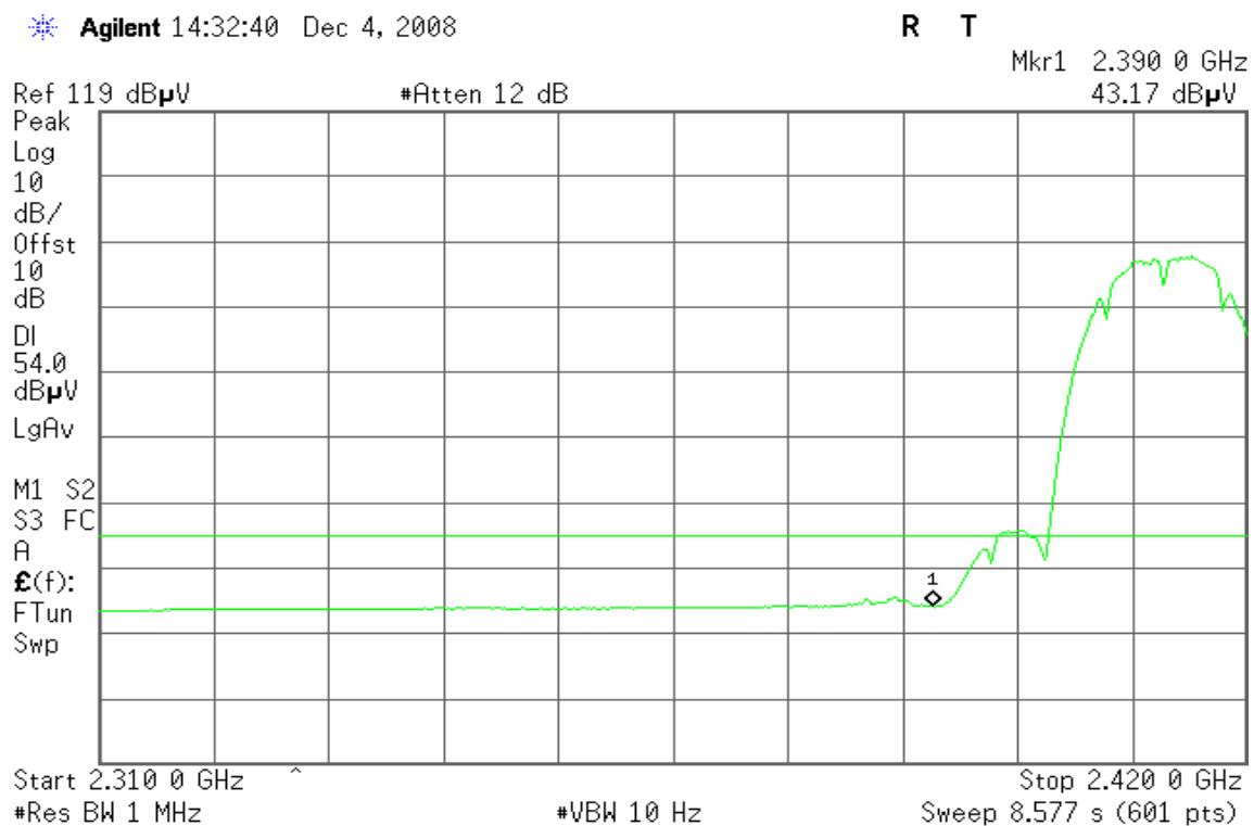
**Band Edges (IEEE 802.11b / CH High)****Detector mode: Peak****Polarity: Vertical**
