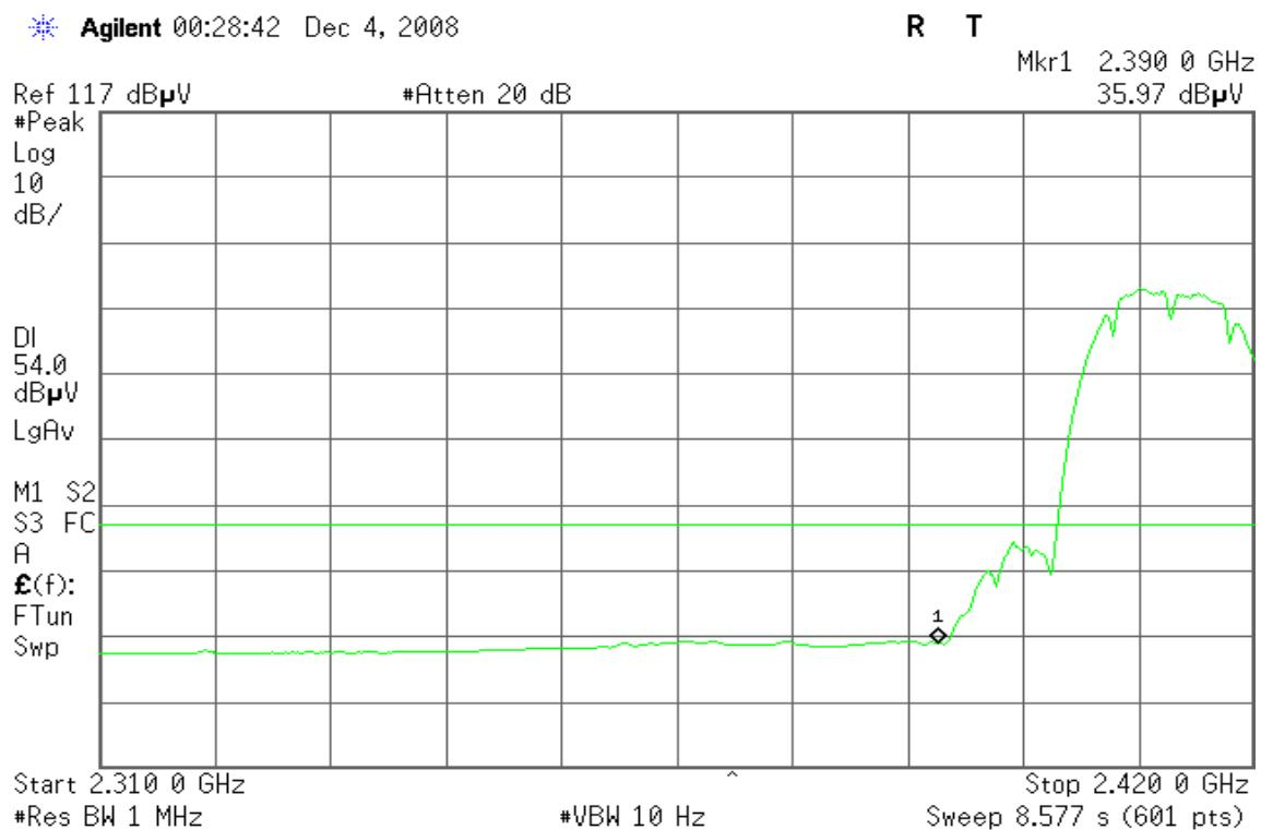
**Band Edges (IEEE 802.11b / CH High)****Detector mode: Peak****Polarity: Vertical**
