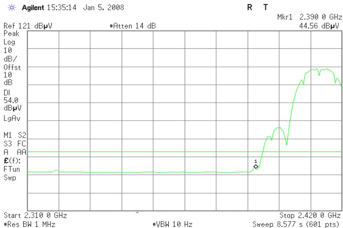
**Band Edges (IEEE 802.11b / CH High)****Detector mode: Peak****Polarity: Vertical**
