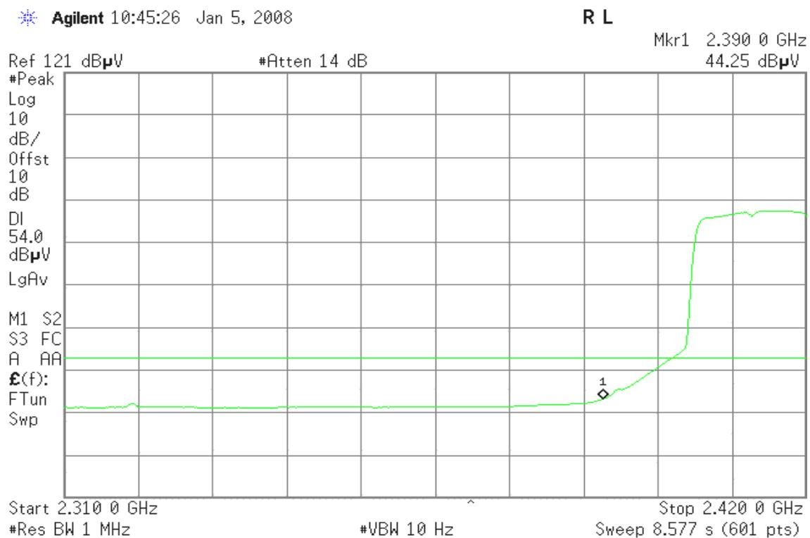
**Band Edges (IEEE 802.11g / CH High)****Detector mode: Peak****Polarity: Vertical**
