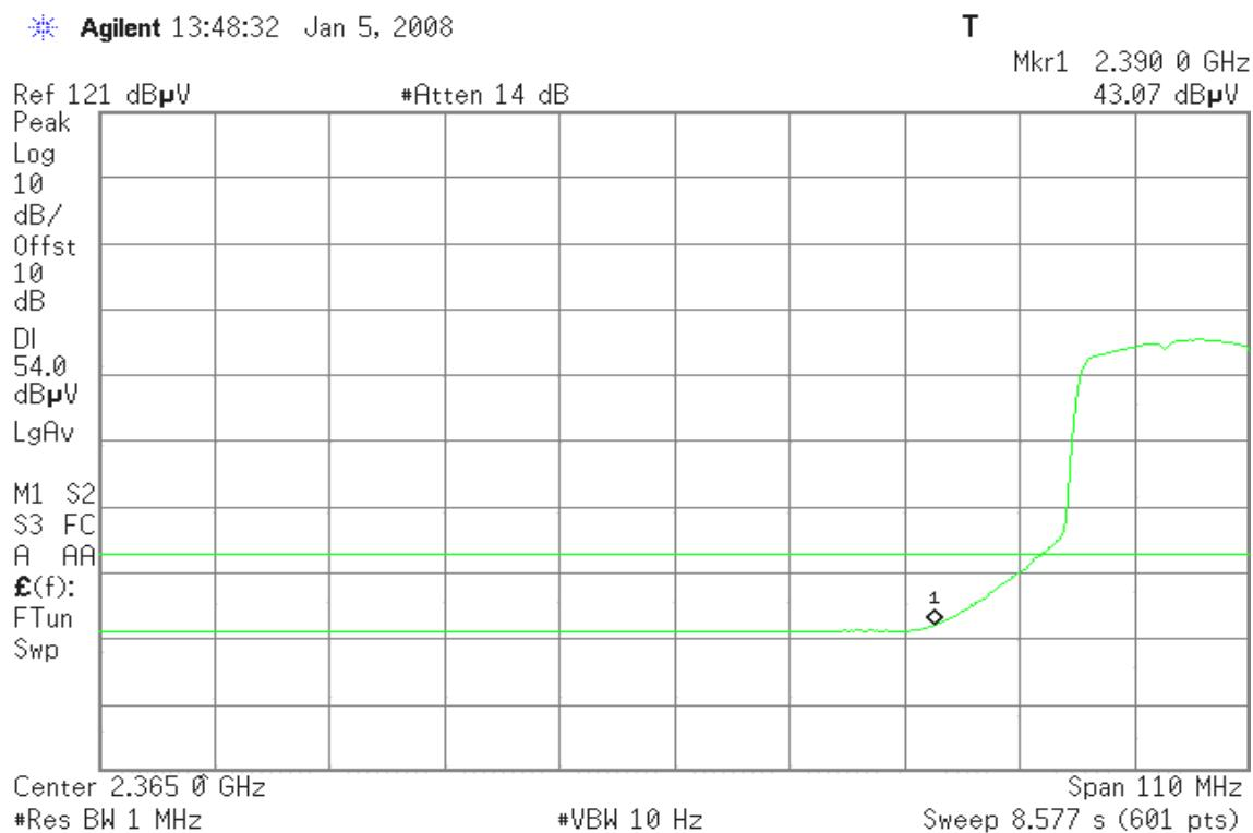
**Band Edges (IEEE 802.11g / CH High)****Detector mode: Peak****Polarity: Vertical**
