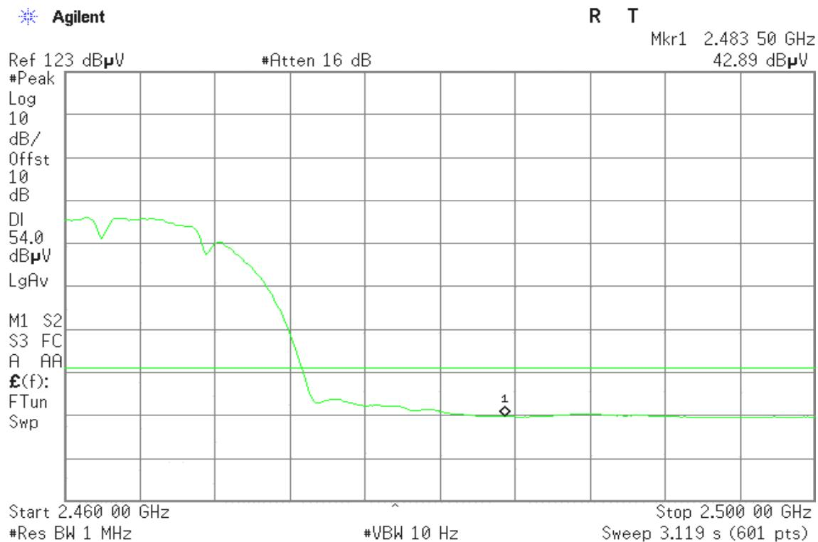
**Band Edges (IEEE 802.11g / CH Low)****Detector mode: Peak****Polarity: Vertical**
