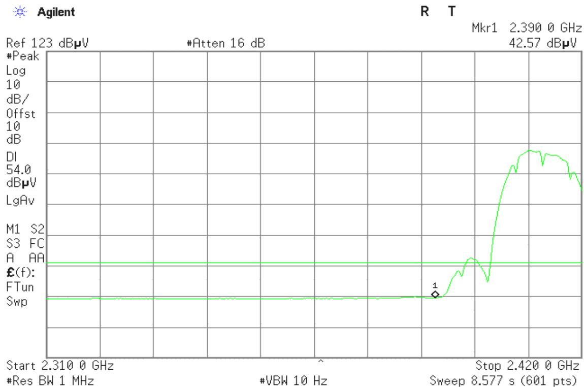
**Band Edges (IEEE 802.11b / CH High)****Detector mode: Peak****Polarity: Vertical**
