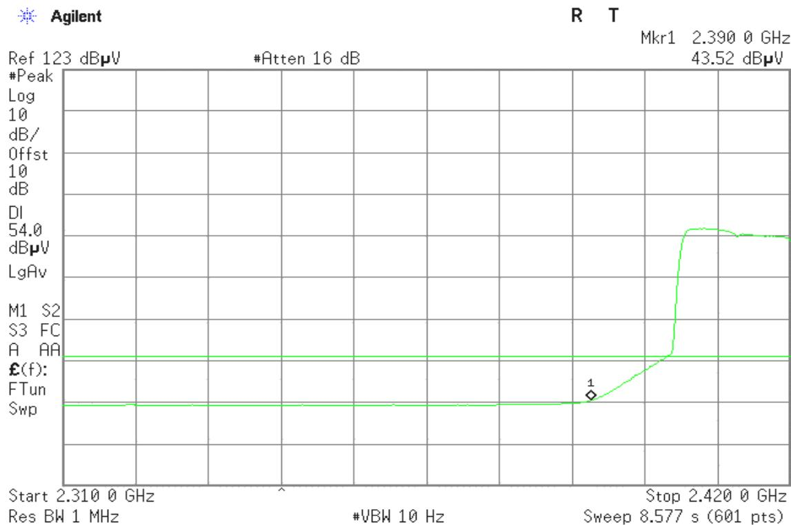
**Band Edges (IEEE 802.11g / CH High)****Detector mode: Peak****Polarity: Vertical**
