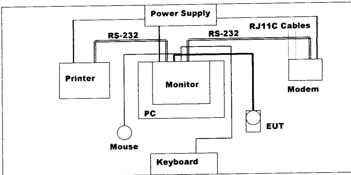
During testing the EUT(PC Camera)r) was connected to video port of Grand Video Capture Card. So there is need for additional grand video capture card. The EUT's PS2 connector was connected to the PS/2 port. A modem was connected to the series port and a printer was connected to the parallel port. Two telephone line(RJ11C cables) connected to the Phone Jack of modem and the Line Jack of modem. A keyboard and mouse were connected to the PS/2 port.
