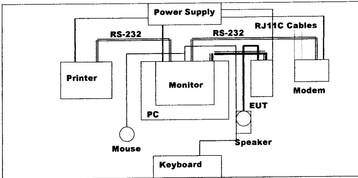
During testing the EUT(External CD-ROM) was connected to Compaq PC's SCSI I/O port. So there is need for additional SISC Card. A speaker was connected to audio jack of EUT. A modem was connected to the series port and a printer was connected to the parallel port. Two telephone line(RJ11C cables) connected to the Phone Jack of modem and the Line Jack of modem. A keyboard and mouse were connected to the PS/2 port.
