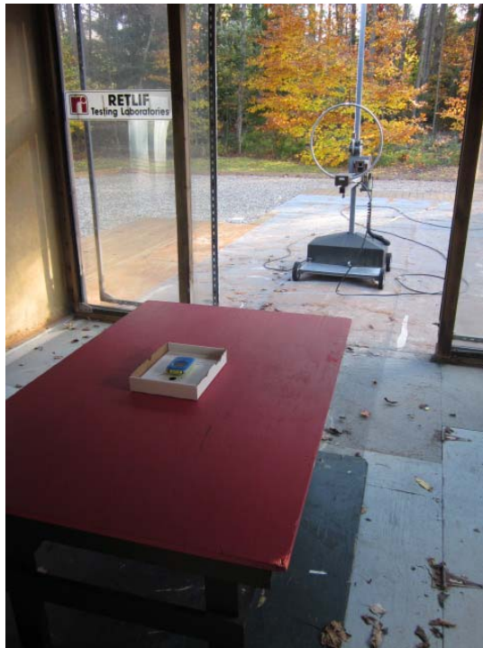
Test Setup, Fundamental and Spurious Emissions, 450 kHz to 30 MHz
