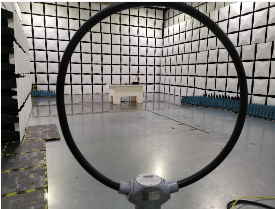
Photograph 2: EUT Test Setup in the anechoic chamber SAC5, Radiated interference field strength measured at 8
