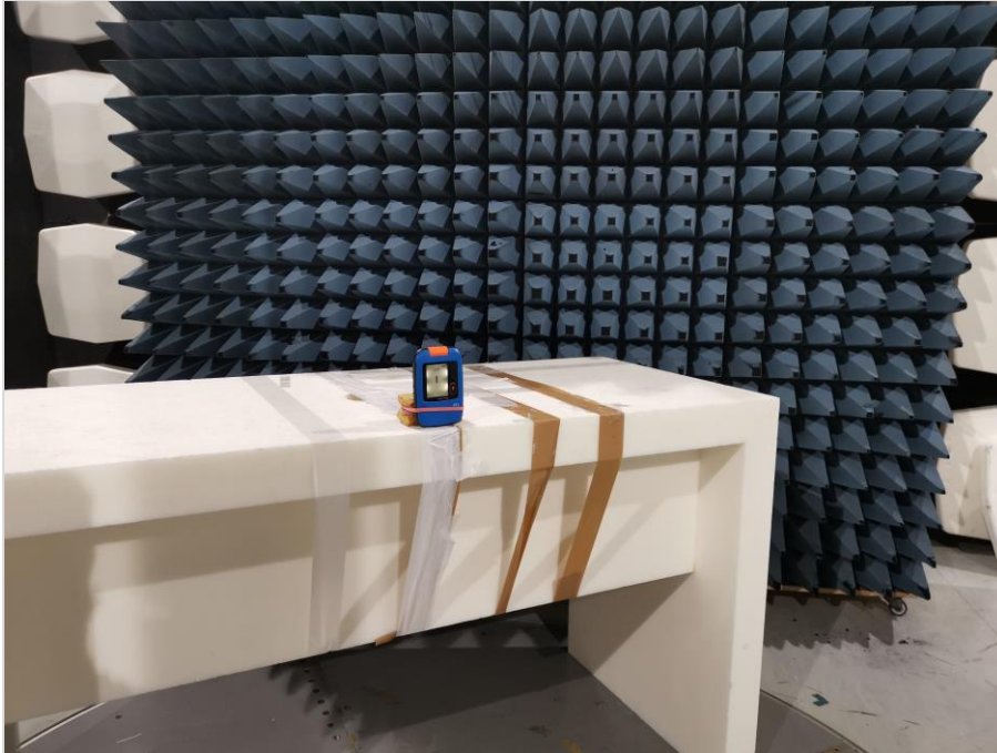
Photograph 5: EUT Test Setup in the anechoic chamber SAC1, Radiated interference field strength
