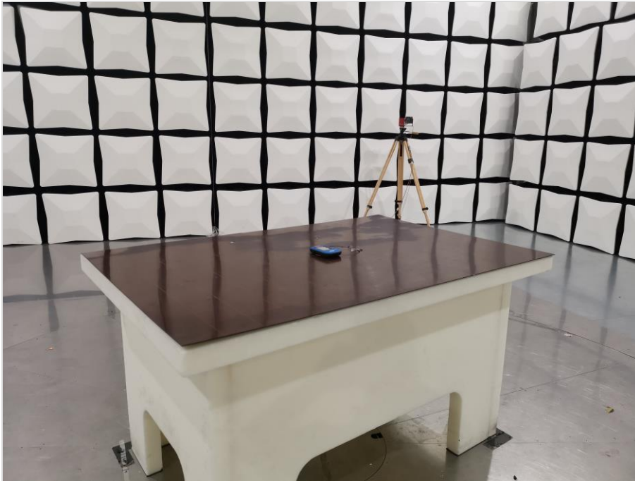
Photograph 1: EUT Test Setup in the anechoic chamber, Radiated interference field strength
