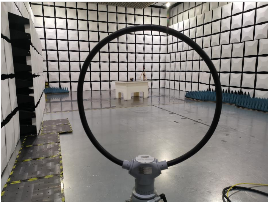
Photograph 2: EUT Test Setup in the anechoic chamber, Radiated interference field strength
