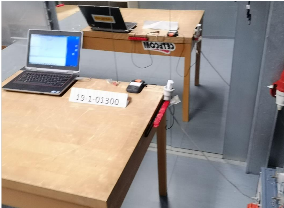
Photograph 9: EUT Setup Conducted emissions on AC-Power lines
