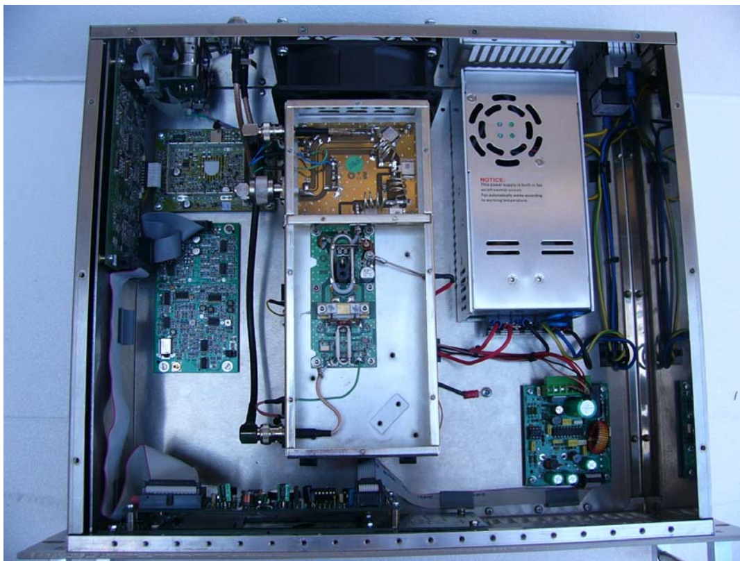
Top without main cover and RF Amp cover
