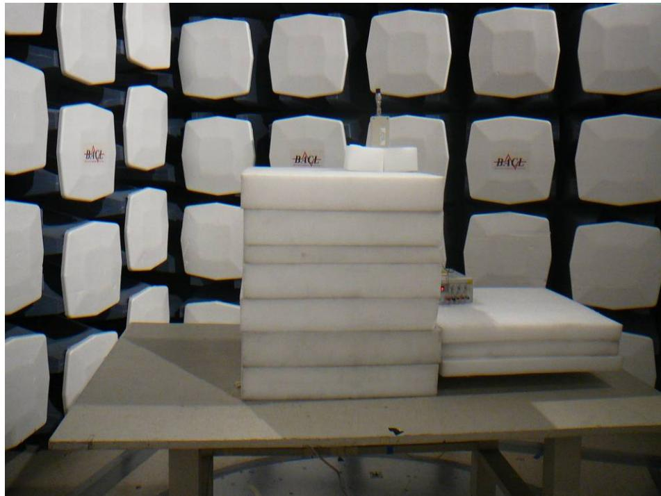
**13.8 Radiated Emission below 1 GHz – Rear View (Z orientation)**
