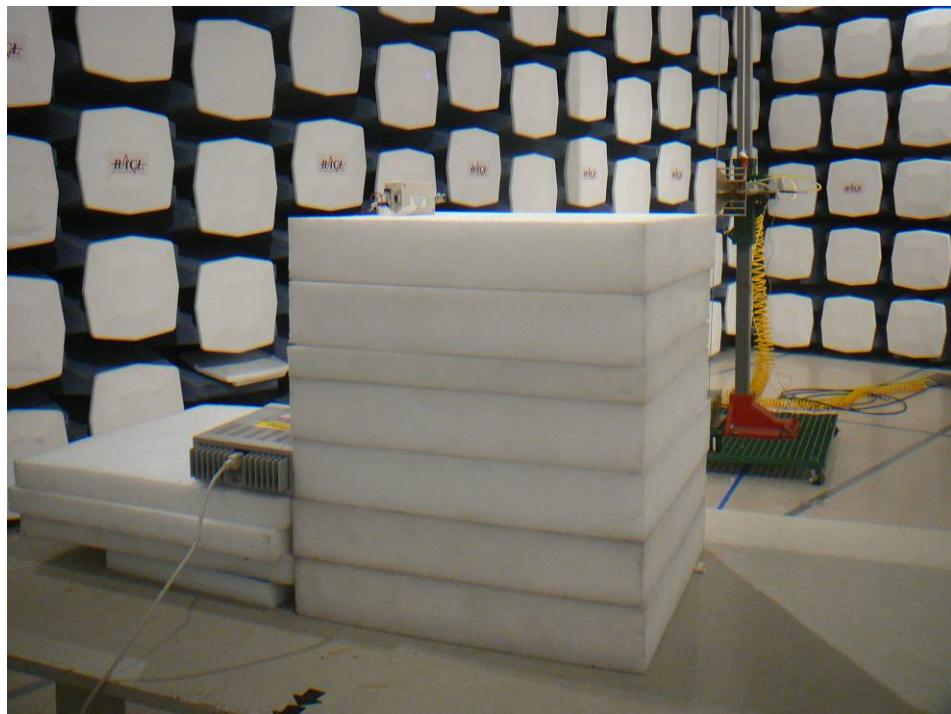
**13.7 Radiated Emission – Front View (Z orientation)**
