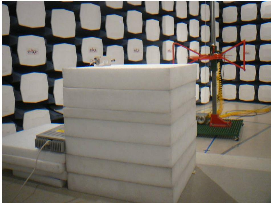
**13.6 Radiated Emission above 1 GHz – Rear View (Y orientation)**
