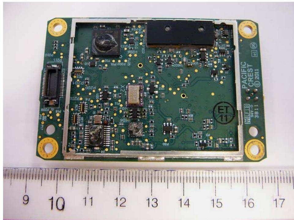
**14.11 Test Supporting Host PCB Board Top View**
