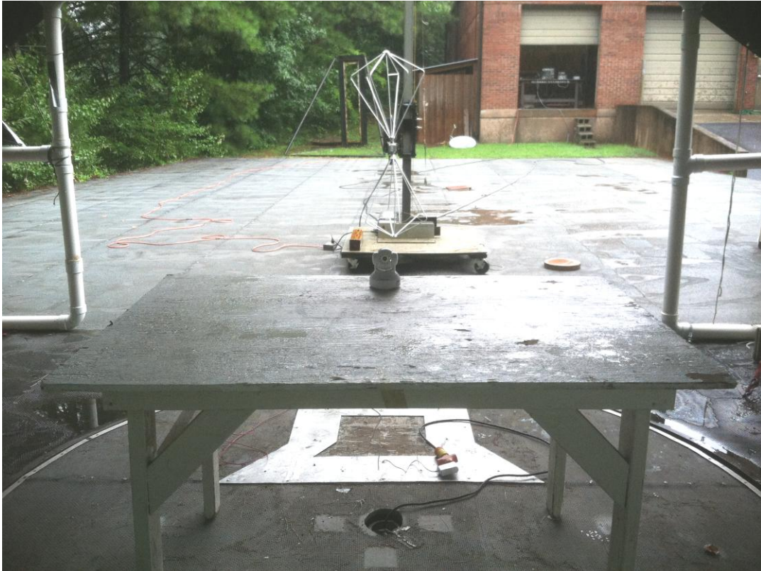
Figure 3. Radiated Emissions 30 MHz - 200 MHz
