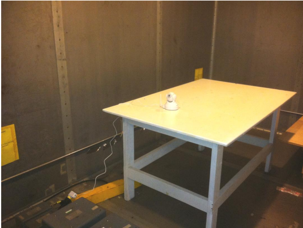
Figure 1. Conducted Emissions Test Setup
