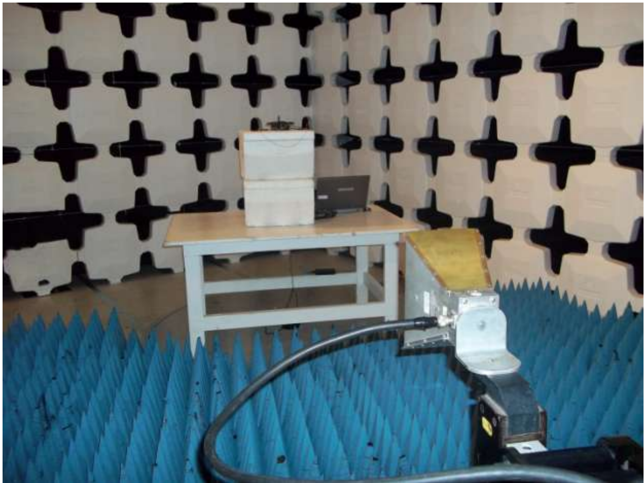
Figure 6. EUT above 1 GHz Test Configuration (Intentional Emissions)
