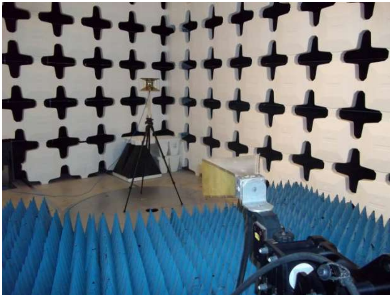
Figure 11. Substitution Testing above 1 GHz
