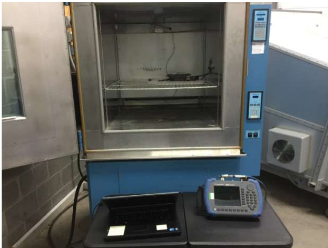
Figure 7. Frequency Stability Test Setup
