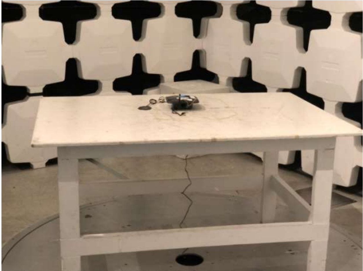
Figure 1. Radiated Emissions Test Setup, Close-Up
