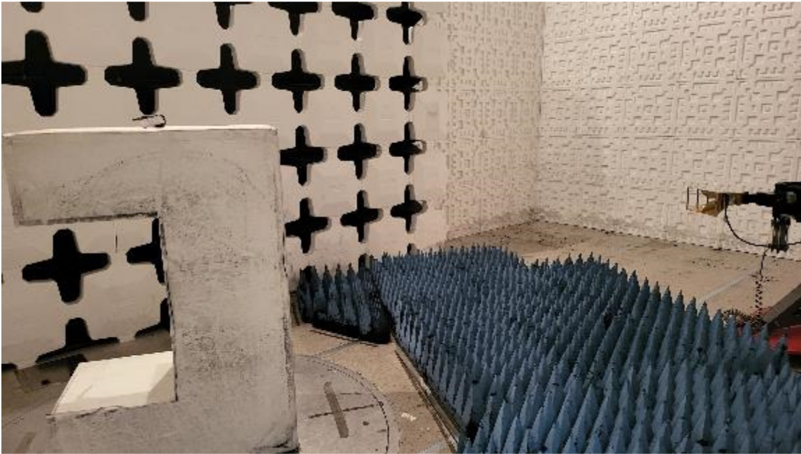
Figure 5. Radiated Emission Test Setup, above 1 GHz, 1.0-mile (STD00-17812)
