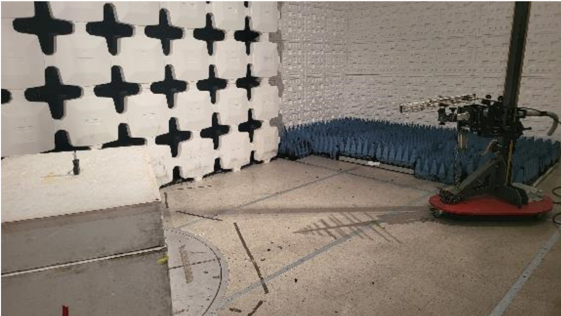
Figure 4. Radiated Emissions Test Setup, 200 MHz to 1GHz, 1.0-mile (STD00-17812)
