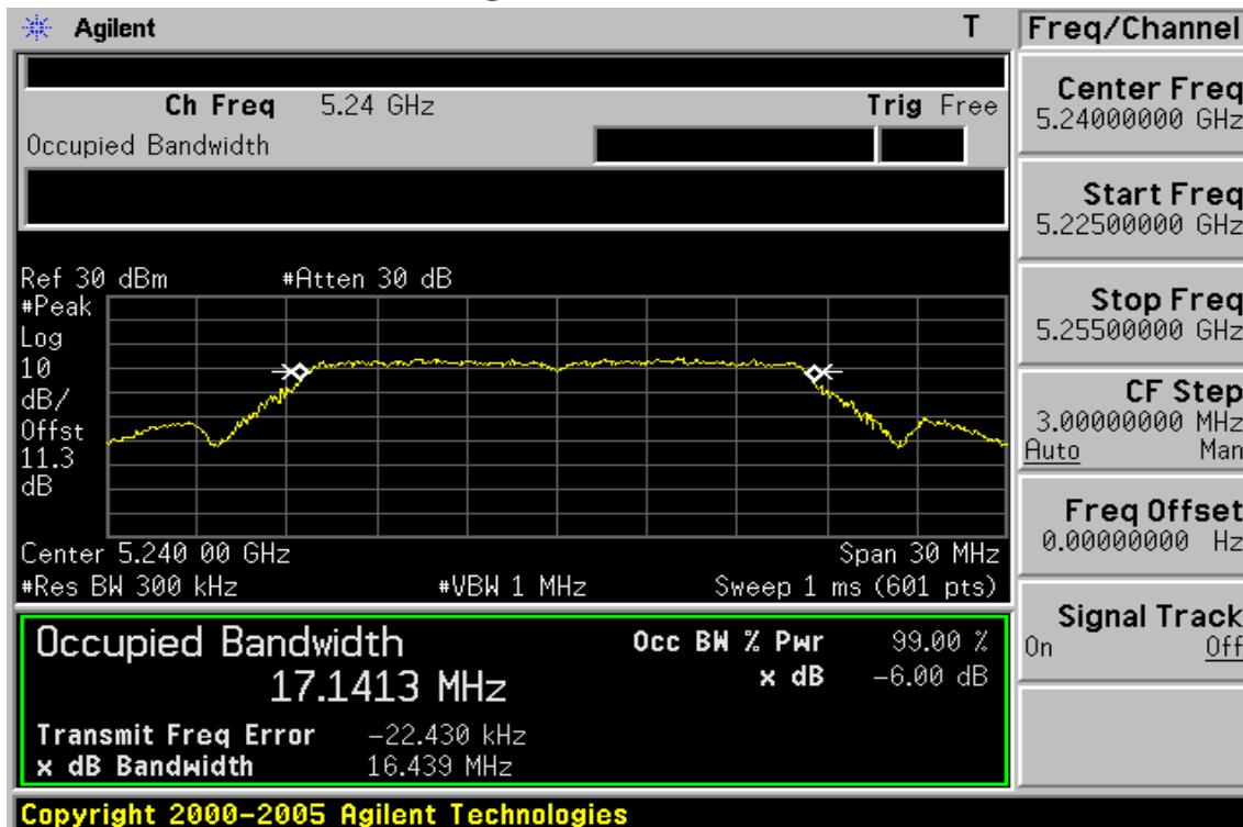
**802.11a, 5250~5350 MHz****99% Band Width Test Data CH-Low (5260MHz)**
