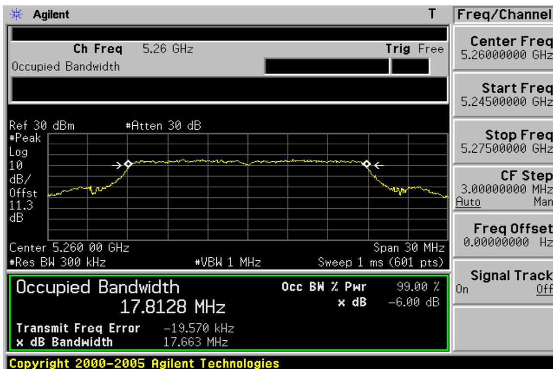
**99% Band Width Test Data CH-Mid (5300 MHz)**
