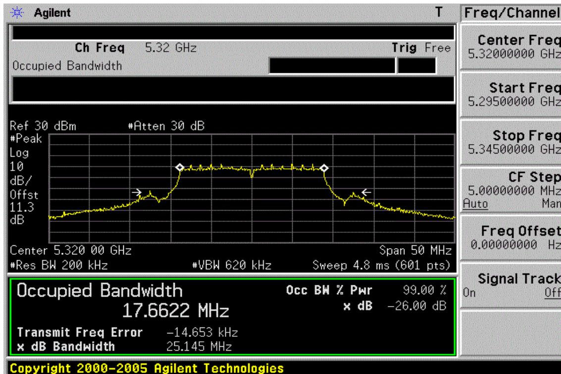
**802.11n HT20, 5470~5725 MHz****26dB Band Width Test Data CH-Low (5500 MHz)**
