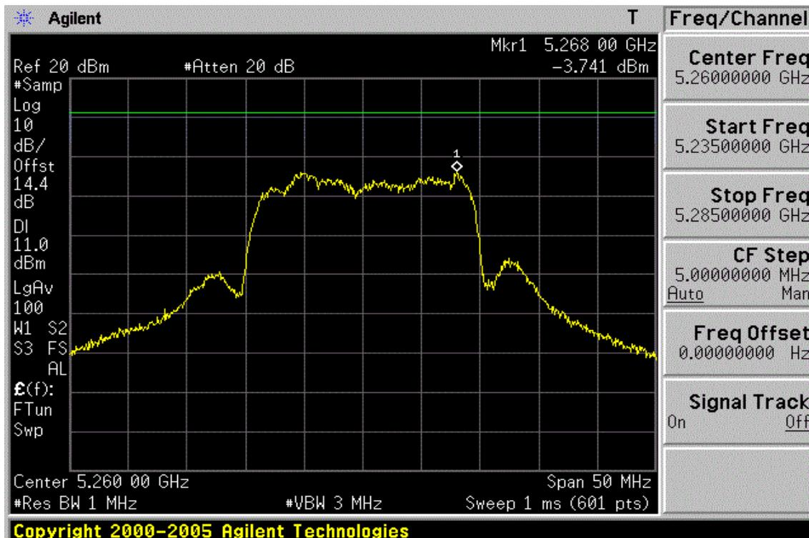
**Peak Power Spectral Density Data Plot (CH Mid 5300 MHz)**
