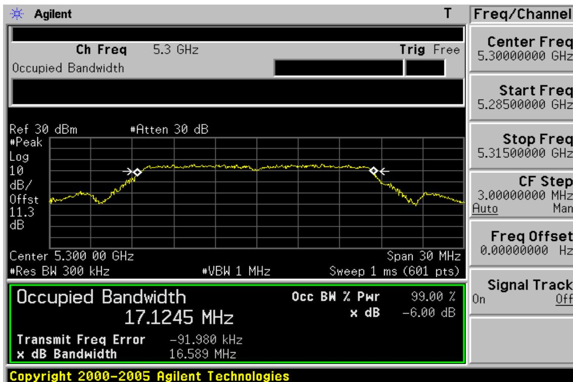
**99% Band Width Test Data CH-High (5320MHz)**
