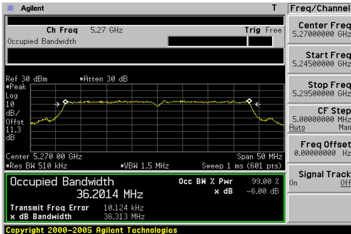
**99% Band Width Test Data CH-High (5310MHz)**
