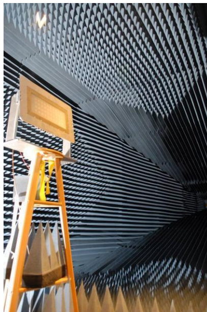
Figure 12 Interior View of the Full Anechoic Chamber
