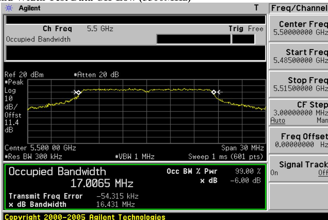
**99% Band Width Test Data CH-Mid (5580MHz)**
