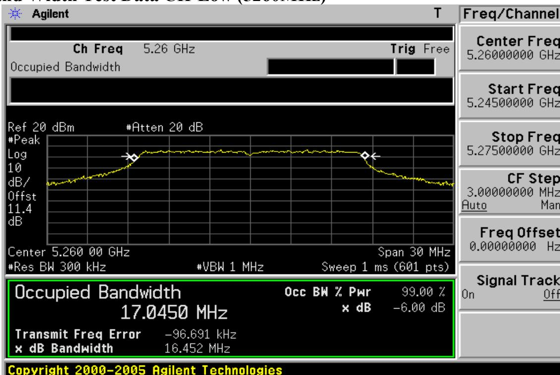
**99% Band Width Test Data CH-Mid (5300MHz)**
