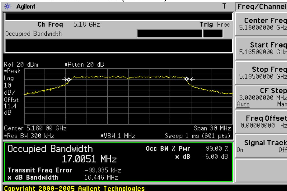
**99% Band Width Test Data CH-Mid (5220MHz)**
