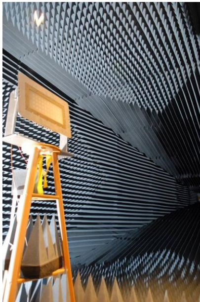
Figure 12 Interior View of the Full Anechoic Chamber
