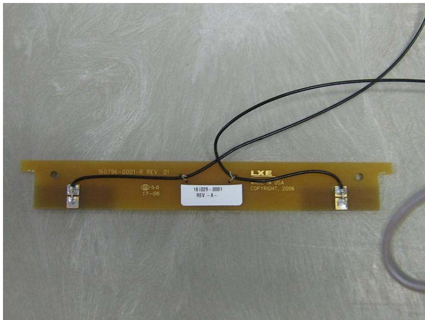
802.11b/g antenna removed from interior of dome casing (Closer Look)
