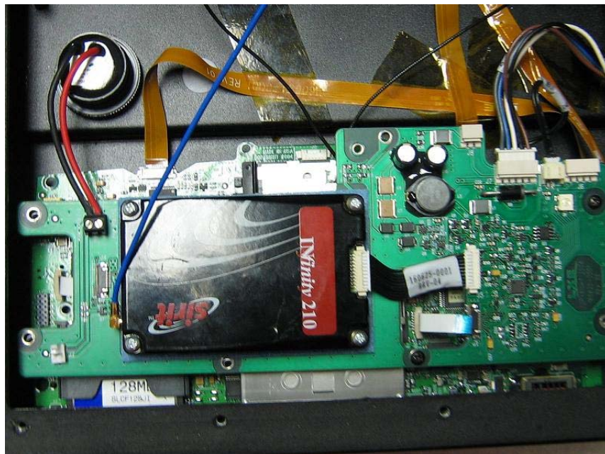
Top Board ( RFID reader) & Bottom Board ( 802.11b/g) Installed
