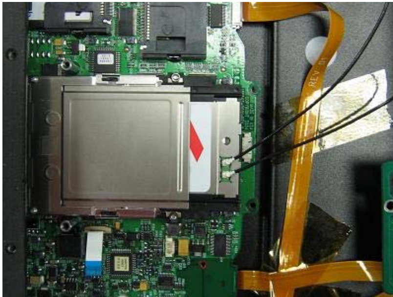
Bottom Board - 802.11b/g installed Dual UFL connectors
