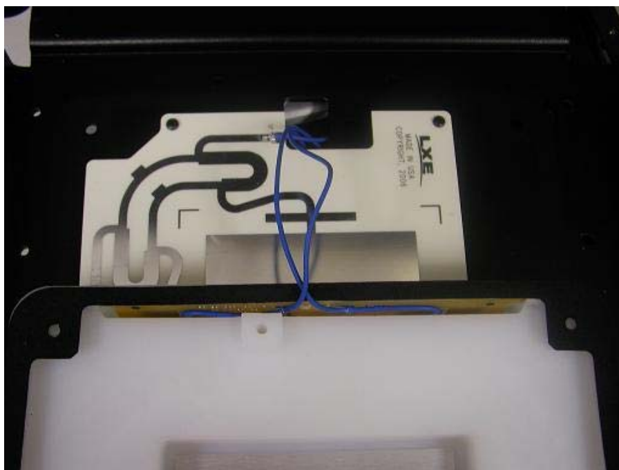
Antenna Dome attachment to Module
