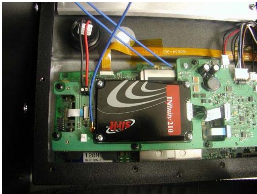
RFID Module Mounting in RX2
