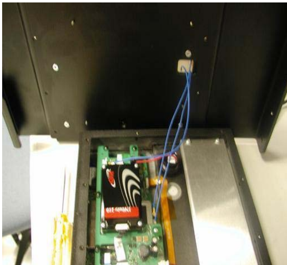
RFID Module with cable throughput attached to Antenna
