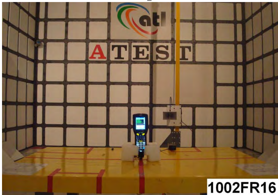
Description : Front View of Radiated Emission Test _ Above 1GHz
