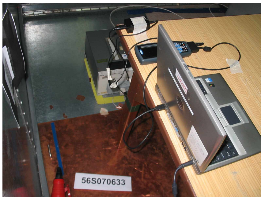
Conducted Emissions Test Setup - AC Mains (Rear View)
