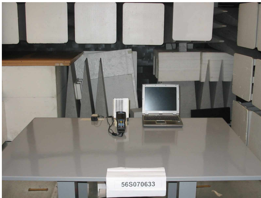
Radiated Emissions Test Setup (Front View)
