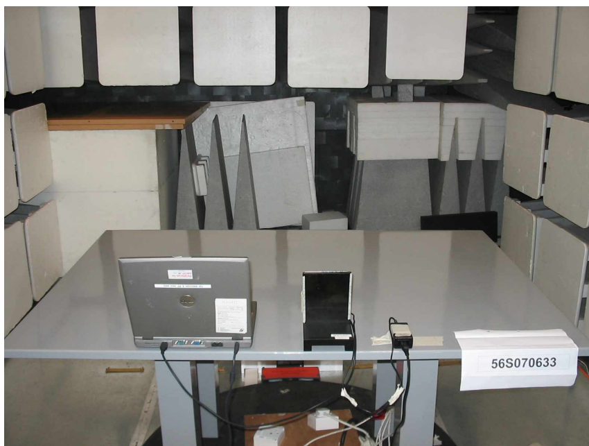
Radiated Emissions Test Setup (Rear View)
