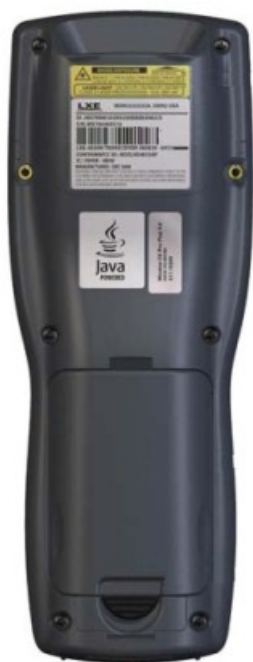
Figure 1 CDRH / IEC 825 Caution Label Location – MX8, Back
