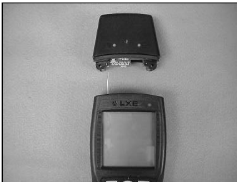
Figure 4: Endcap removed, exposing omni antenna
