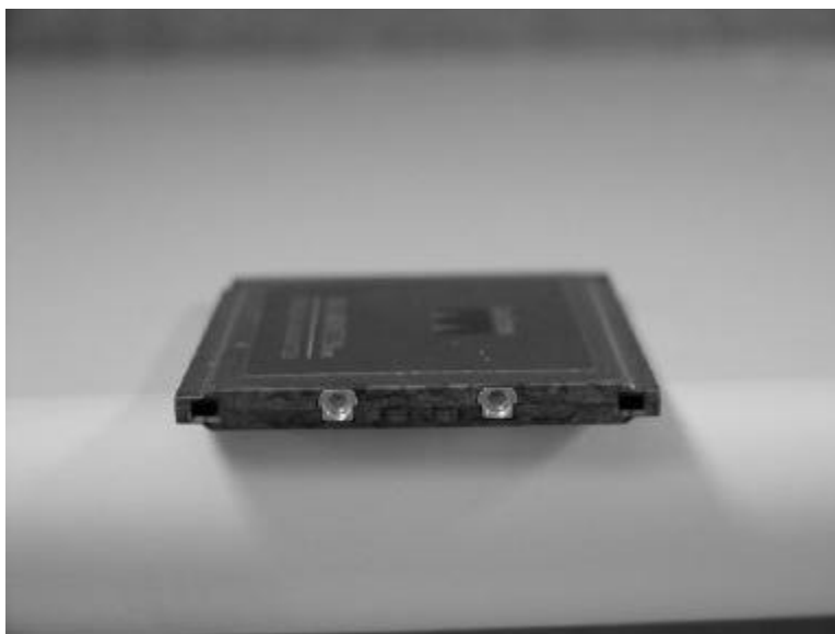
Figure 2: View of antenna connector
