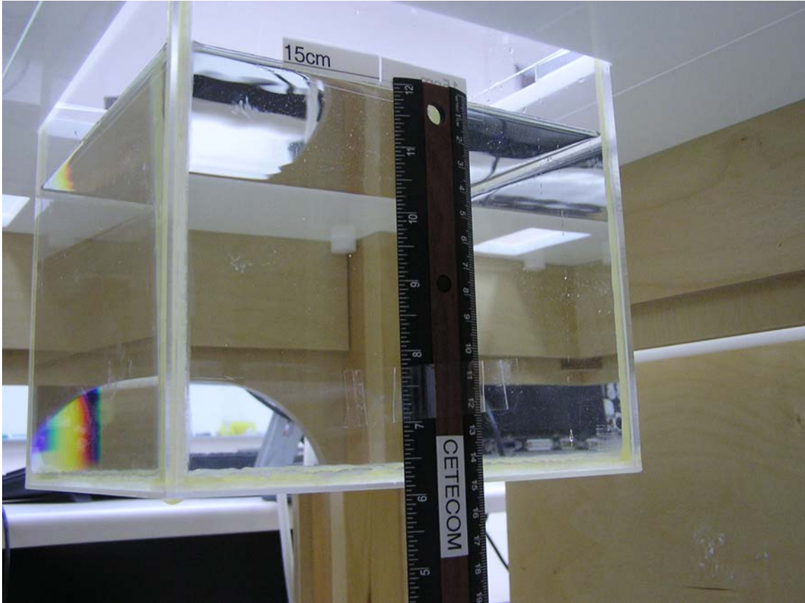
Photo 5. Photo to demonstrate 15 cm Z-axis flat phantom
