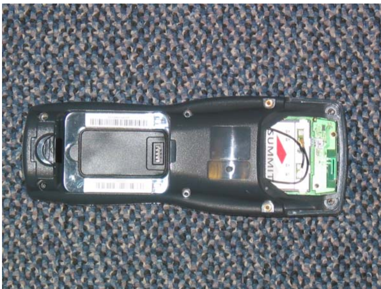
Back of Device with Top Cover Removed With Bluetooth
